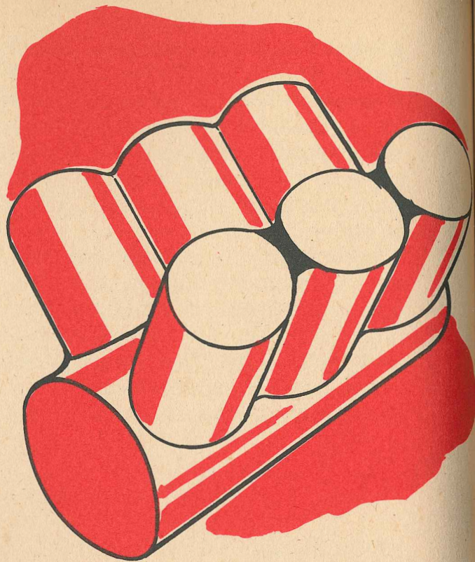
Cylinders arranged in a V-formation in a six-cylinder engine.
